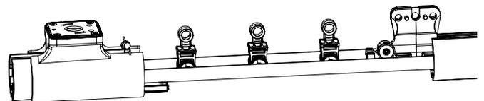
Install the Drive Pulley into the H-Rail Track and install the Pendant into the attachment tab.
