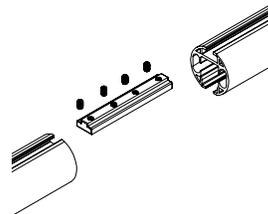
Step 3. Spray both sides of the H-Rail Track with silicone.
