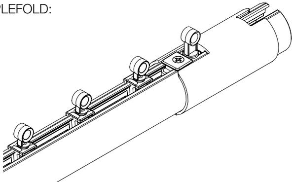
Step 31. Install the Pendants and End Caps or Finials onto the Drive and Return Pulleys.
