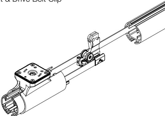
Step 11. Pull the Master Carrier Body through the R-TEC Track and assemble the Drive Pulley onto the H-Rail Track.
