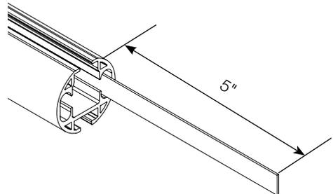
Step 15. Mark the Drive Belt tooth at the edge of the Track.
