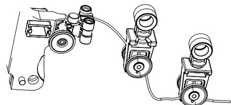
Step 28. Install the Master Carrier and Carriers into the Track.
