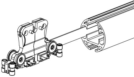
Step 8. Remove the Master Carrier Body and Drive Belt Clip.
