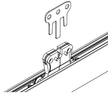
NOTE: The Master Carrier should move freely back and forth.
