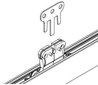
Step 26. Remove 1 Ripplefold Carrier from the end that's closest to the Return Pulley. Leave the cord as shown with the attachment tab exposed.
