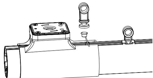
Step 19. Install the Pendant into the End Stop.
