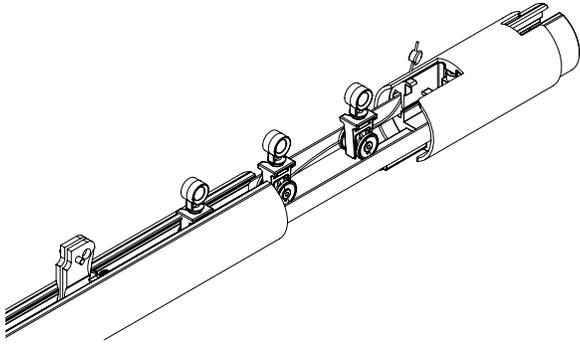
Step 29. Bring both Master Carrier Body halves together and insert the Master Carrier center metal clip.
