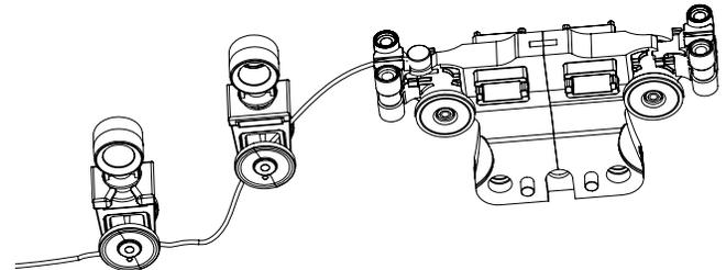
Install the Master Carrier Body and required number of Carriers into the H-Rail Track.
