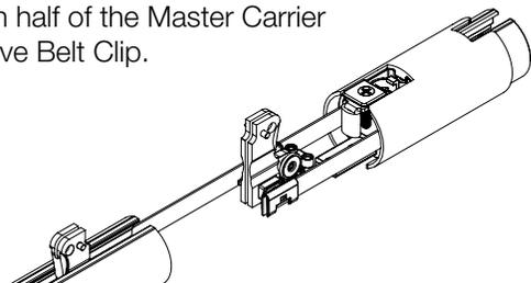
Step 24. Bring both Master Carrier Body halves together and insert the Master Carrier center metal clip.
