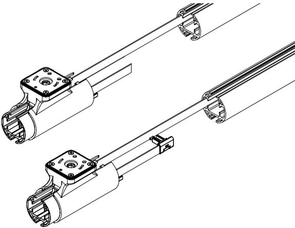
Step 10. Attach half of the Master Carrier Body to the Drive Belt & Drive Belt Clip
