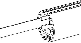
Step 9. Install the Drive Belt through the Drive Pulley, then install the Drive Belt to the Drive Belt Clip.
