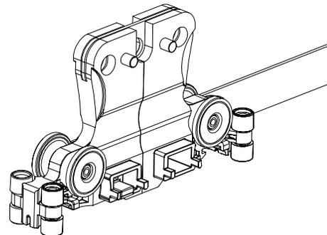
Step 7. Pull the Master Carrier Body through the H-Rail Track.
