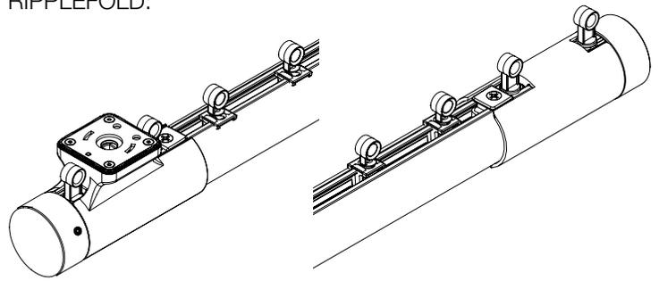
Step 32. Install the Master Carrier Arms onto the Master Carrier Bodies.
