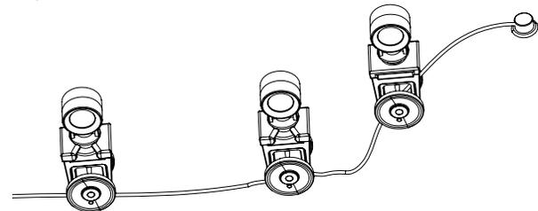
Install the attachment tab into the Master Carrier Body.
