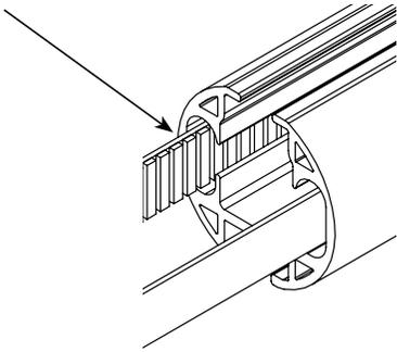
Step 16. Install Drive Belt Clips on both sides of the marked Drive Belt tooth.
