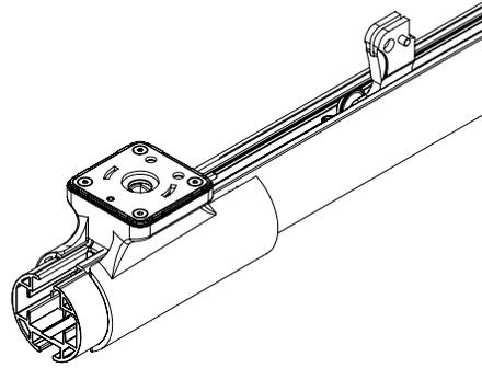
Step 12. Align the Master Carrier Body half to the end of the Track. Cut Drive Belt to length: 5" from end of the Track.
