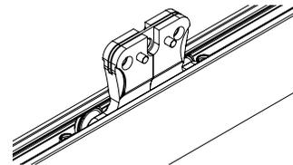
Step 25. Remove the Master Carrier center metal clip.
