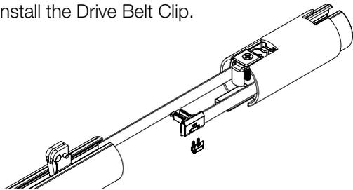
Step 23. Attach half of the Master Carrier Body to the Drive Belt Clip.
