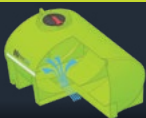
Cutaway shows full drain sump
